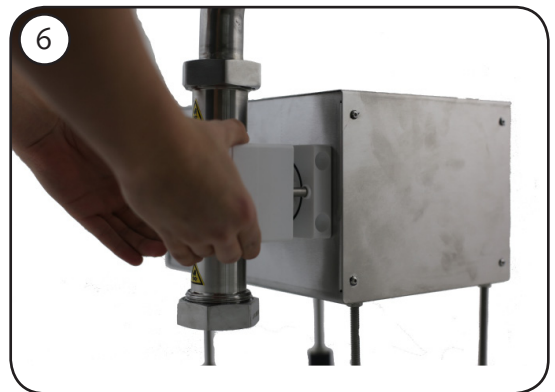
Pull the pump head off by grapping onto the sides and pull towards you.
