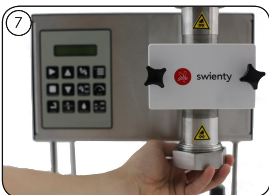
When the machine has stopped dripping, mount the cutoff mechanism. Can be mounted first but not with very viscous liquids. See page 16.
