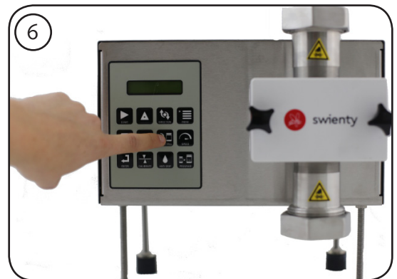
Press the button [Fill/Pump] to change from pump to fill.
