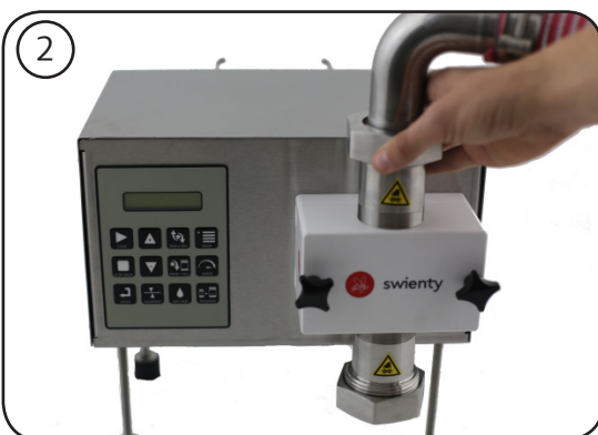
Loosen the valve on top of the pump head to bring in some air. Only loosen it a little so the liquid does not run out. Warning: Always unplug the machine before the pump case is dismantled.
